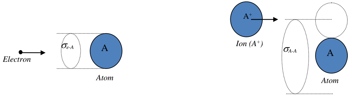
Fig. II-1: Representation of the cross-section in the case where the atom is considered a sphere and without taking into account the interaction potential
