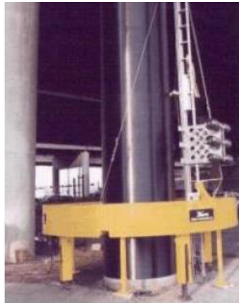
Figure 1.10 : L'enroulement filamentaire [(Master Builders, Inc. and Structural Preservation Systems, 1998) et (Balaguru et al., 2009)].
