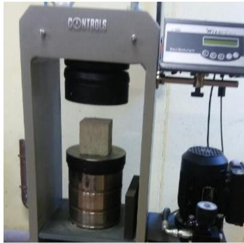
Figure 3.10: Machine de compression.
