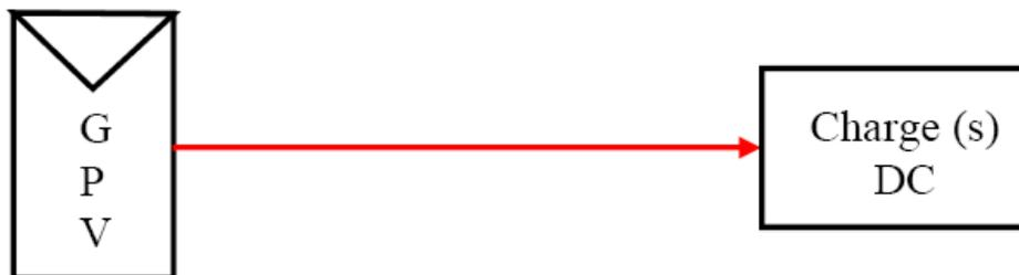
**Figure I.19 Couplage direct GPV-charge.**
