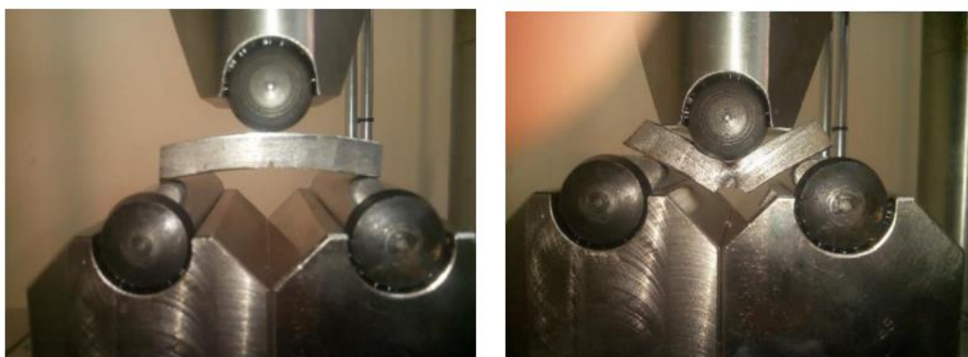
Figure IV. 29. Three point bending test, specimen under test (left), specimen after break (right).
