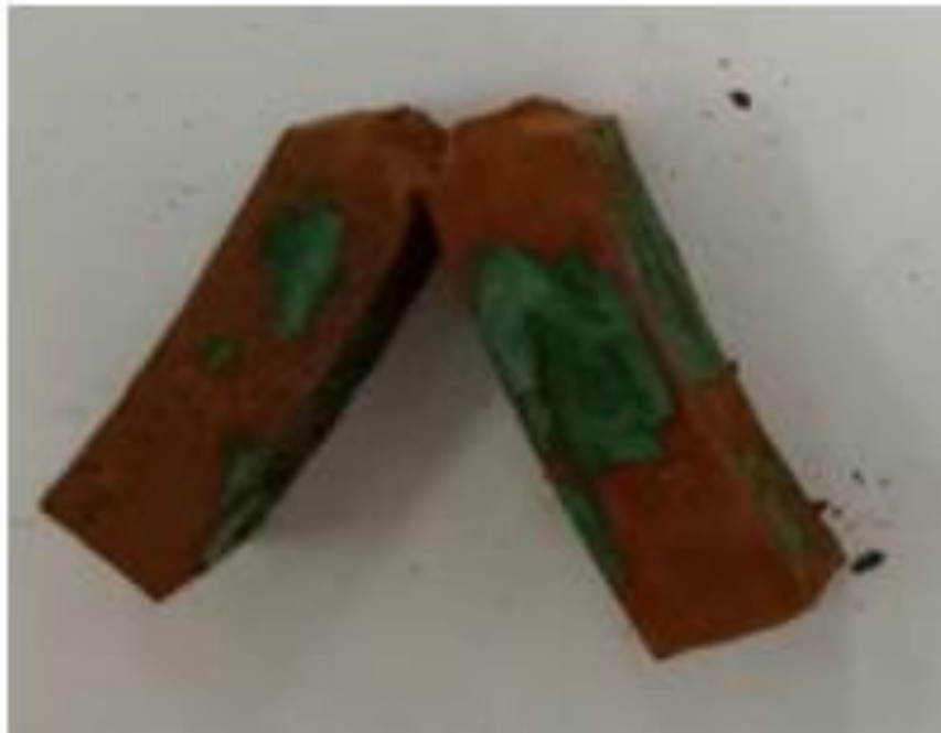
Figure IV. 11. Fractured V-notched Charpy test specimen.
