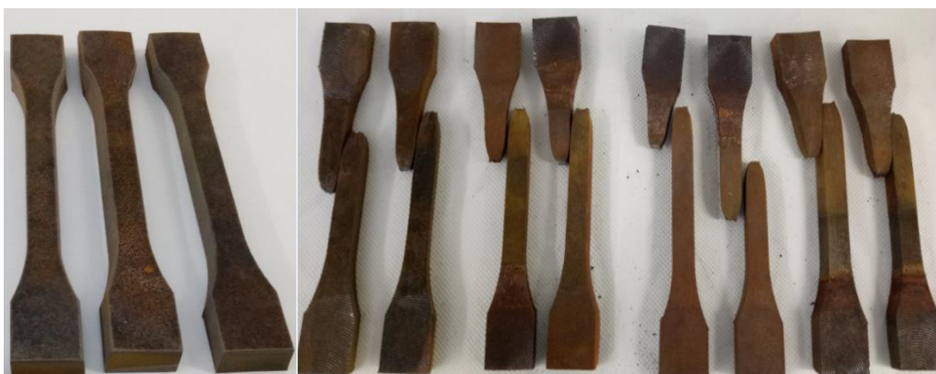
Figure IV. 31. The tensile specimens, before and, after tensile tests.
