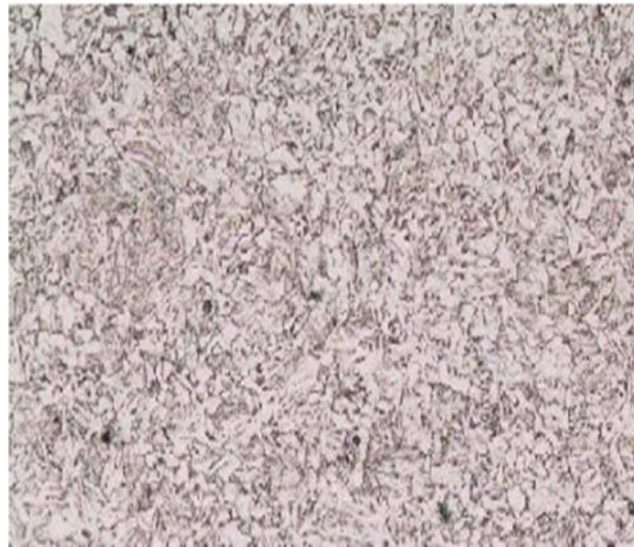
Figure III.5. Microstructure of the pipe section of API 5L X65 steel.
