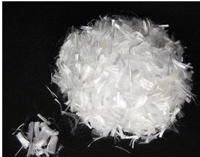
Figure 3.4 – Les fibres PVA (Mavani, 2012).
