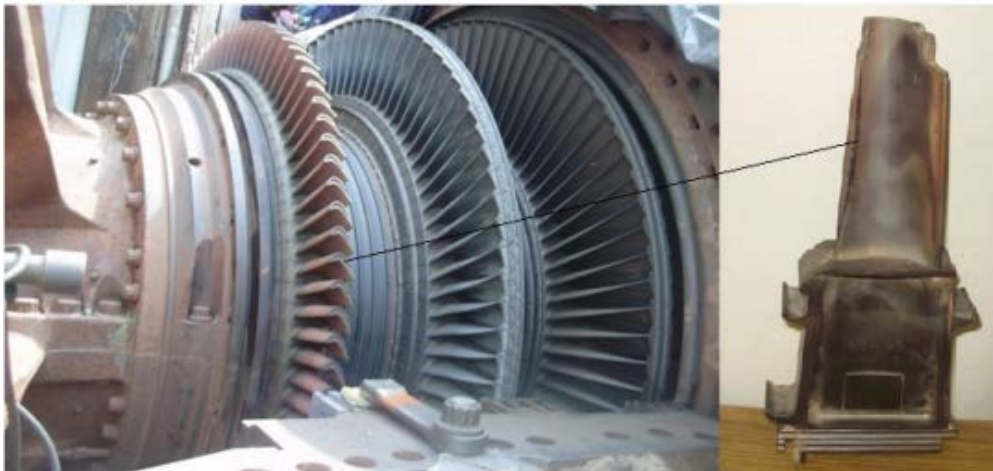
Figure.I.13. (1) Internal view of 30 MW Gas Turbine. (2) First stage Gas Turbine Blade.
