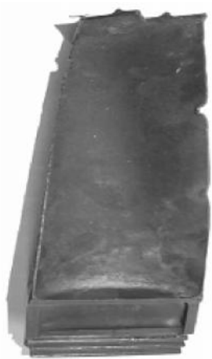
Figure I.19. Blade Geometry and the Firtree Joint of a Damaged Turbine Blade
