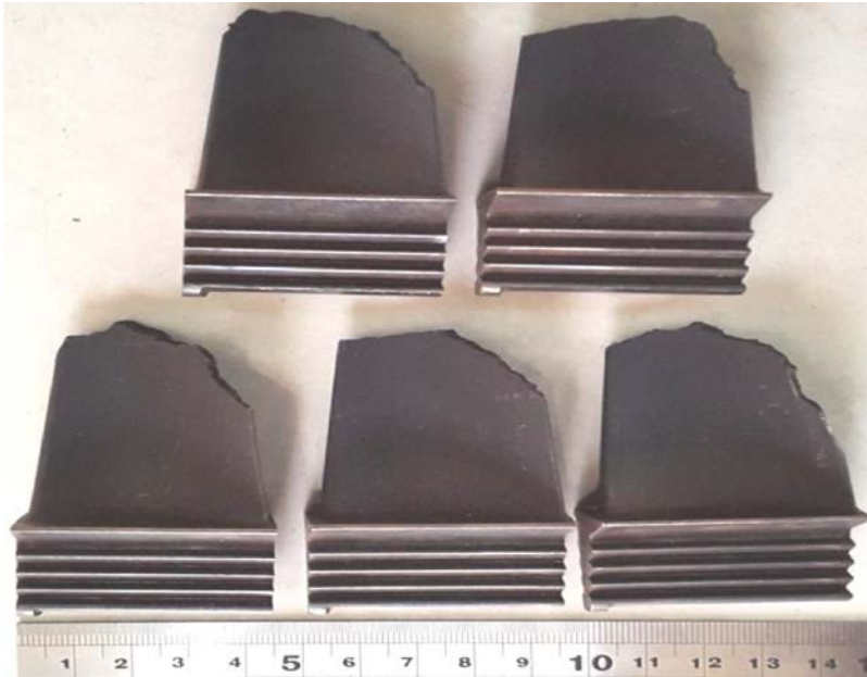
Figure.I.14. Damaged rotor blades of first-stage turbine blades after 6500 h of operation at about 750–800 °C a 6.5 MW gas turbine.
