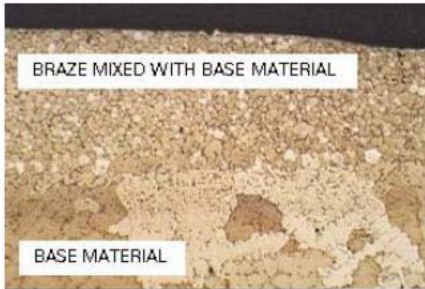
Figure III.45: Overlay brazed Nickel-based Alloy
