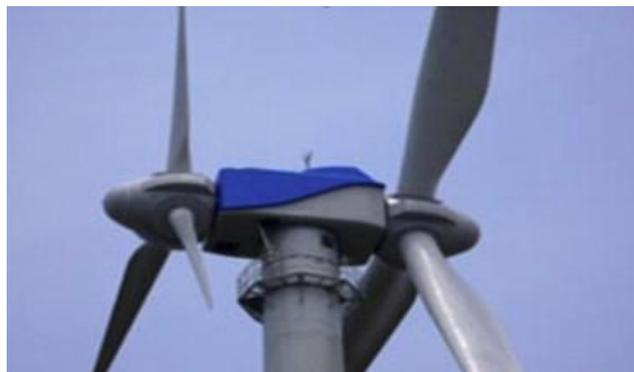
Figure I-14 : Eolienne double rotor.
