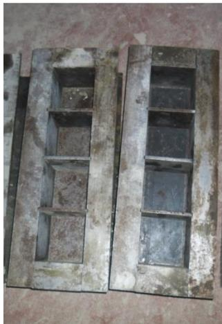
b) Eprouvettes cubiques 100x100x100 mm (compression + abrasion)
