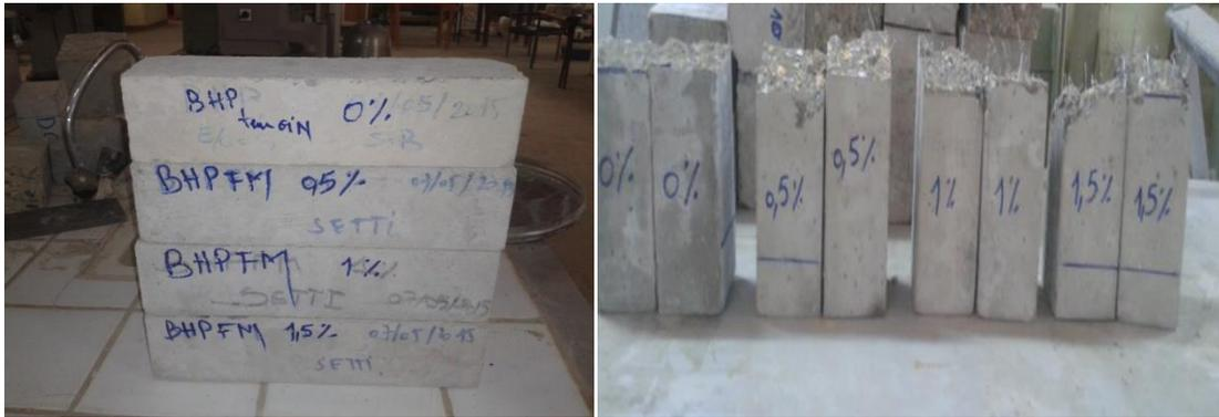
Figure 3.14: Mode de rupture.
