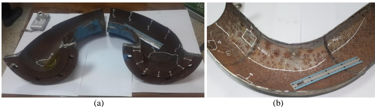
Figure IV.4: General view of the internal surface of failed pipe elbows, (a) elbow I, and (b) elbow II.
