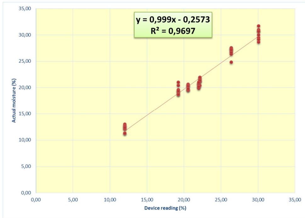
Fig.3. 24 : Calibration curve of the moisture meter PMS 710.
