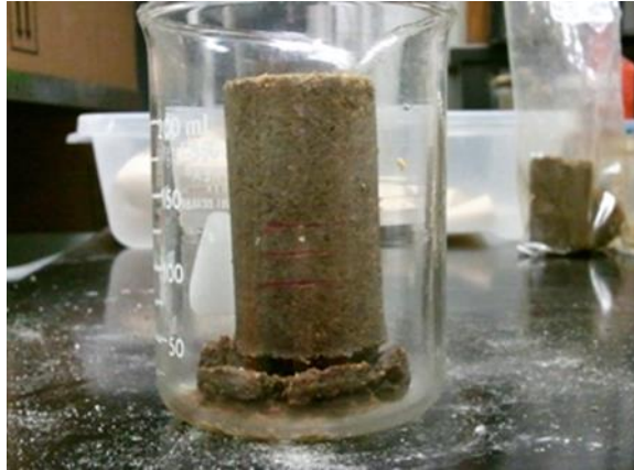
Figure 4. 30- (CB80 B 20) Partially Soaked in water exposed to high temperature
