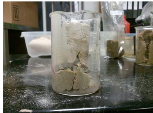
Figure 4. 27- (S80 B 20) Partially Soaked in Water
