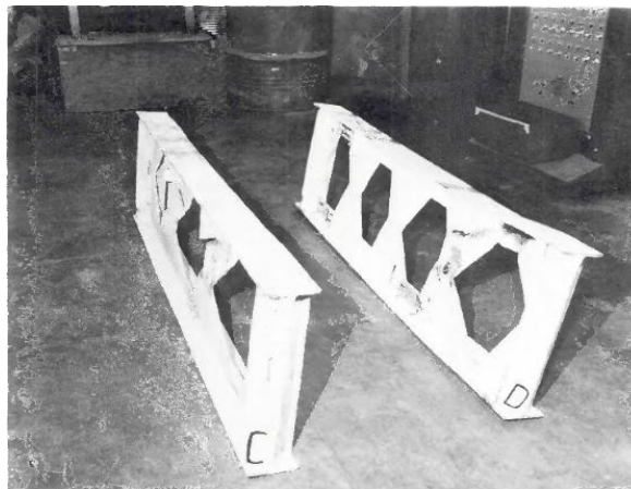
Figure 1-15. Web-post crippling due to compression [65].
