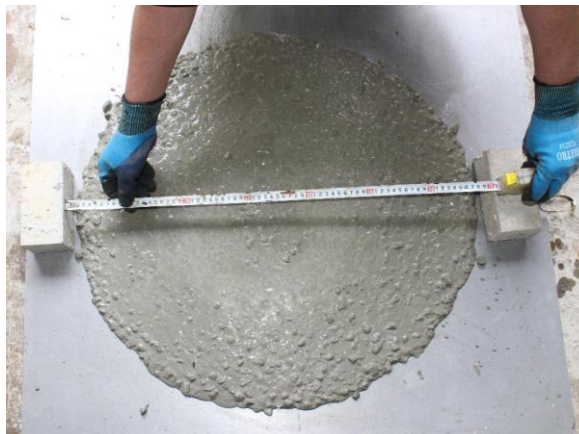
Figure 2.6. Essai d'étalement (Flow Test)
