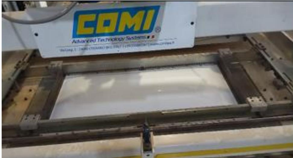
**Figure 1-9 : Sheet bubbling (pre-stretching).**
