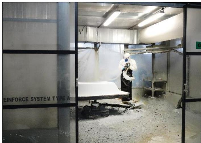
**Figure 1-12 : bathtub reinforcement chamber [44].**
