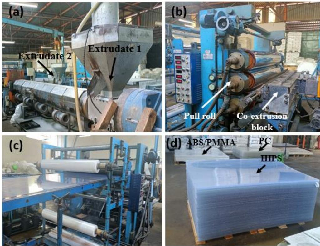
**Figure 3-3: Fabricated polymer sheets via extrusion and co-extrusion processes; (a) single screw extrudates, (b) co-extrusion block and pull roll, (c) extrudate, and (d) extruded polymer sheets.**
