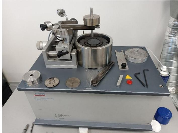
**Figure 3-14: Tribometer measurement device.**
