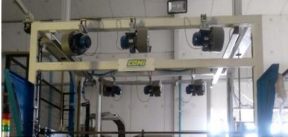
**Figure 1-11 : Fans opened for bath cooling.**
