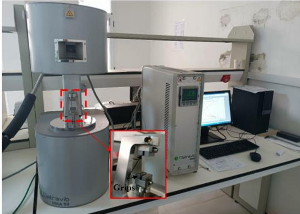
**Figure 3-6: Dynamic mechanical analyzer.**
