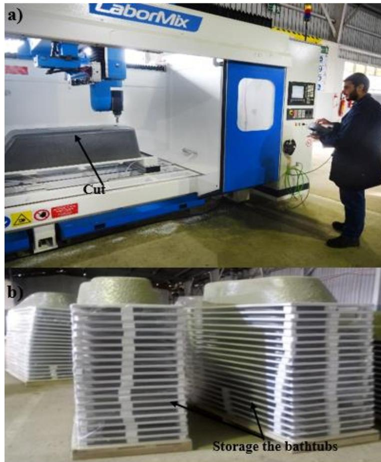
Figure 1-14: a) Bathtub cutting, and b) bathtub storage.
