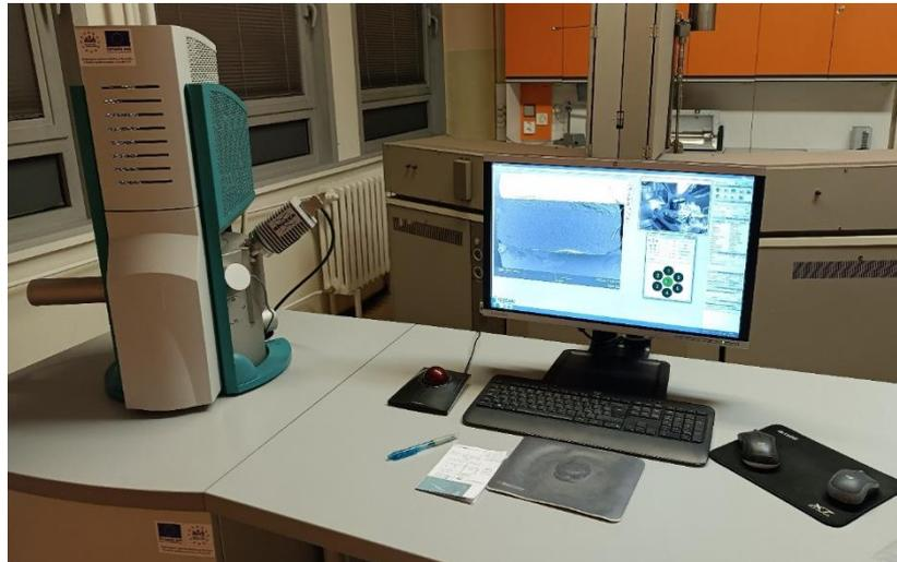
**Figure 3-9: Scanning Electronic Microscopy analyzer.**
