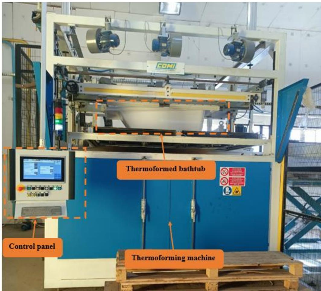
Figure 1-6 : Thermoforming machine used at EIMS Miliana.
