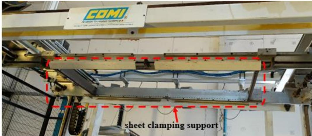
**Figure 1-7 : Sheet clamping system.**
