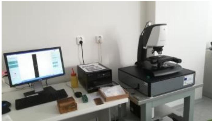
**Figure 3-16: PLu neox 3D confocal microscope profiler [145].**
