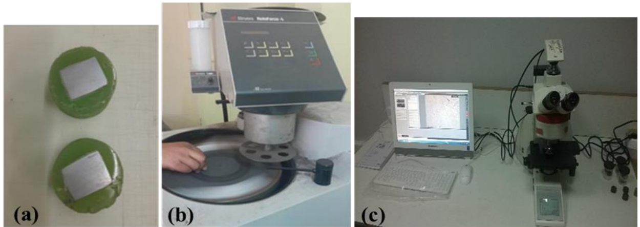
Figure 2-1 : (a) Samples before polishing, (b) Polishing samples, (c) optical microscope<<LEICADM4M>>.
