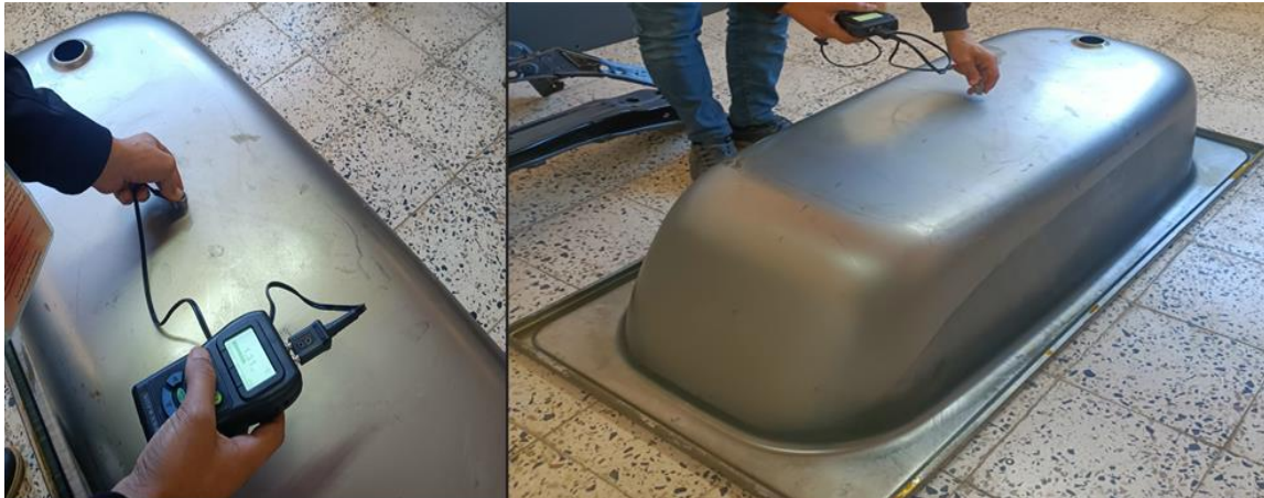
Figure 2-17 : Defect-free bathtub thickness measurement using the Sofranel EHC 09B ultrasonic device.
