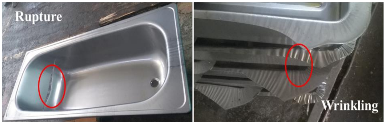
Figure 3-1 : Visual representation of rupture and wrinkling defects in bathtubs manufactured by the EDD process.
