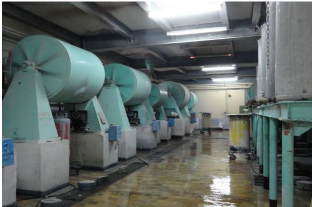
Figure 1-3 : Grinders used at EIMS to grind mass and covering enamel.
