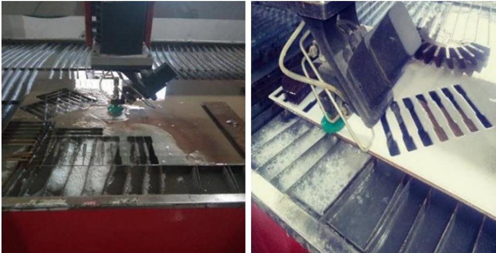
Figure 2-3 : Cutting the test specimens with a water-jet.
