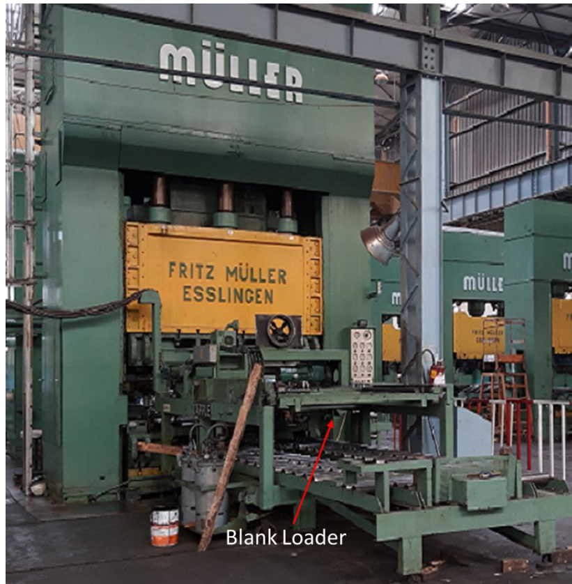
Figure 1-6 : BZE1600-32 press for deep-drawing bathtubs.
