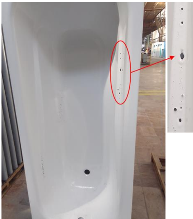
Figure 1-12 : Bathtub with air bubble defects.
