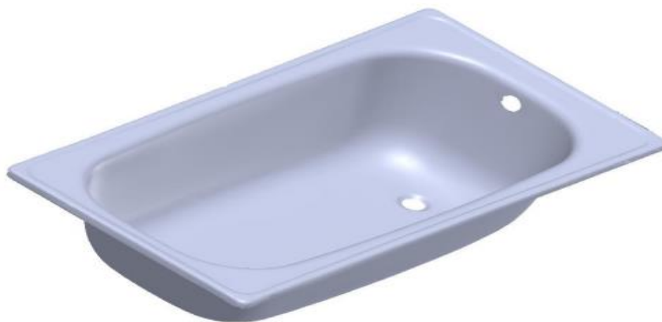
Figure 2-15 : Final CAD shape of the bathtub.
