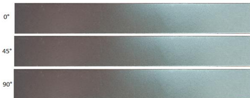
Figure 4-2 : Test samples cut in three directions.
