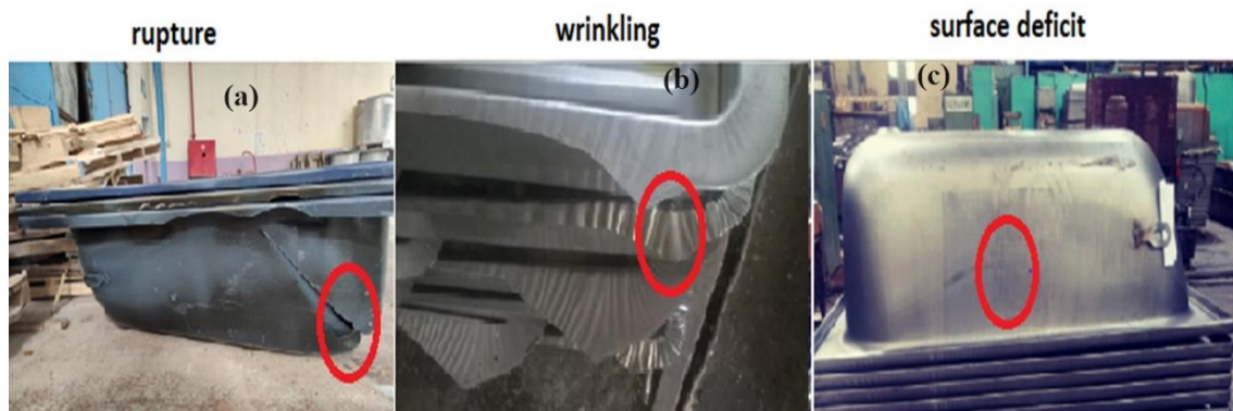
Figure 1-11 : Defects on the bathtubs.
