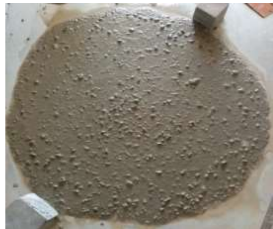
Fig. III.6.b. Spread of mixture for SCC1
