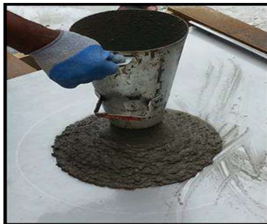
Fig.I.8. Slump flow test
