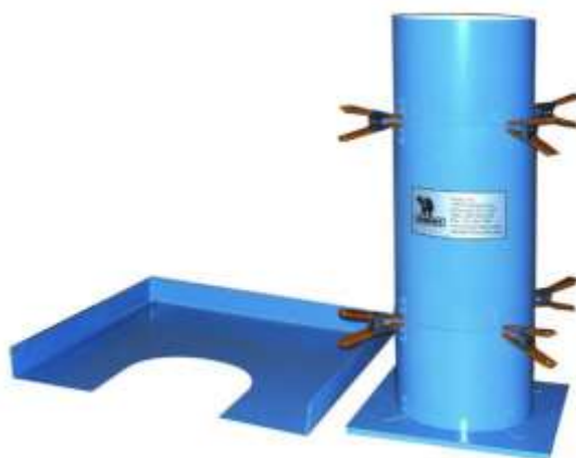
Fig.I.10. Column segregation test
