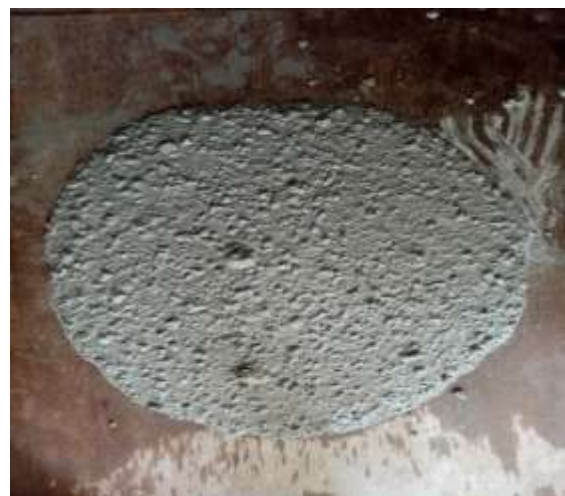
Fig. III.6.f. Spread of mixture for SCC5
