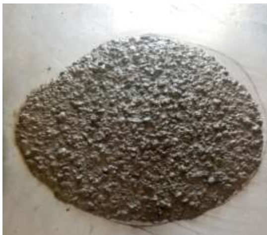
Fig. III.6.g. Spread of mixture for SCC6
