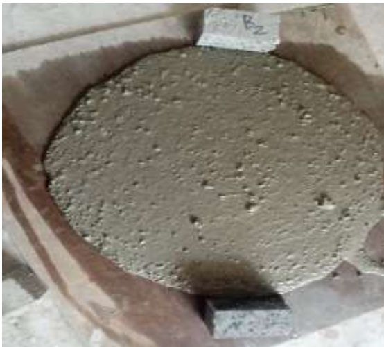
Fig. III.6.e. Spread of mixture for SCC4
