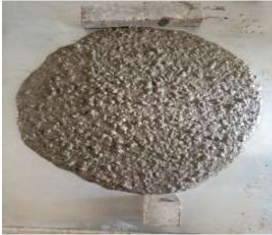
Fig. III.6.c. Spread of mixture for SCC2
