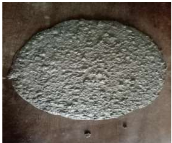
Fig. III.6.h. Spread of mixture for SCC7
