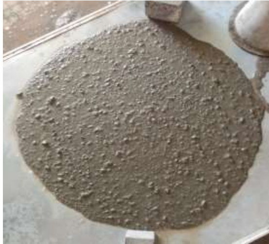
Fig. III.6.i. Spread of mixture for SCC8
