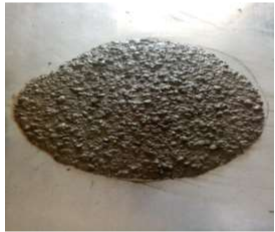
Fig. III.6.d. Spread of mixture for SCC3
