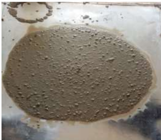
Fig.III.6.a. Spread of mixture of FTM
