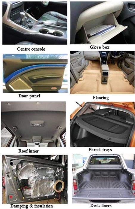
Figure 1.21. Some interior automotive parts made from bio-fiber composites [57].
