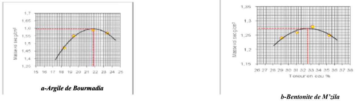
Figure 3. Essai de compactage
