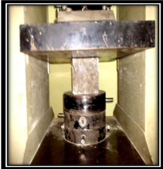
Figure 5.3: Essai de compression sur cube
