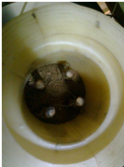
Figure IV-13. View of type of soil–root composite (root distribution form with four roots)
