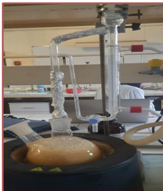
Figure III.8: Clevenger apparatus used for hydrodistillation of ginger essential oil.
