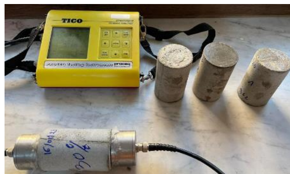
Figure IV. 15 Ultrasonic pulse velocity test
