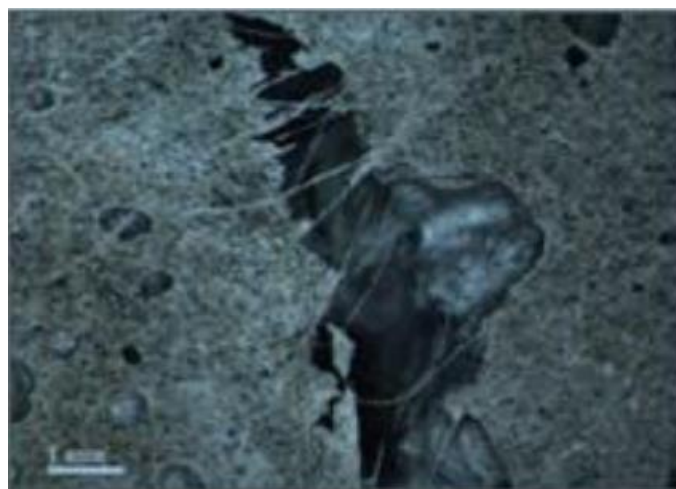
Figure II. 16 SEM (Scanning Electron Microscope) image showing the bridging of cracks by polypropylene fibres [105].
