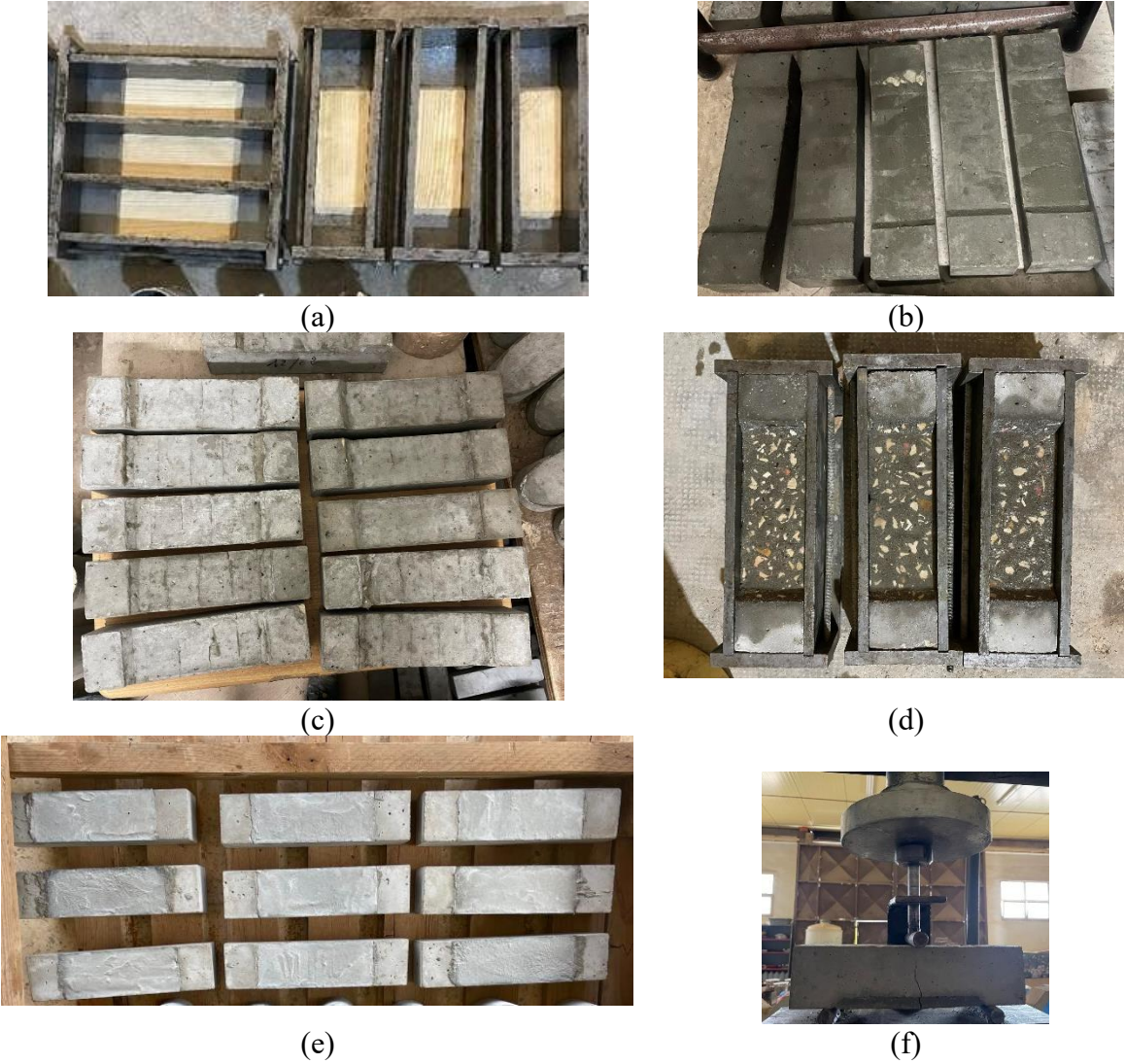
Figure IV. 21 Preparing concrete specimens for compatibility by flexural test.
