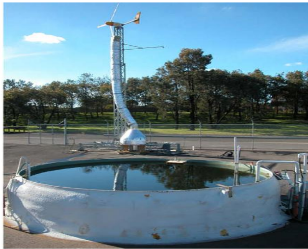
Figure II. 20: Hybrid SCPP and Solar Pond Configuration by Akbarzadeh et al [105].
