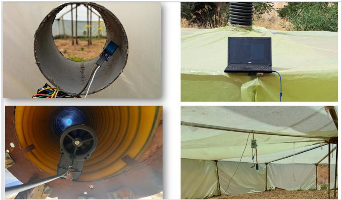
Figure III. 8: Photographic view of the experimental SCPP setup with the installed sensors and instrumentation.
