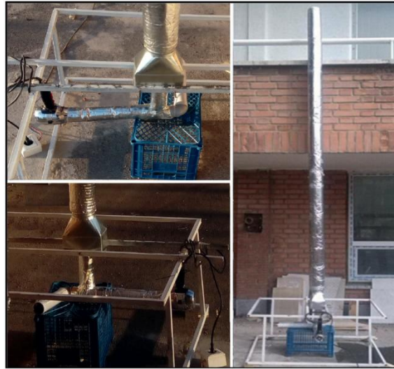
Figure II. 19: Pilot Hybrid SCPP Using Exhaust Gases by Shahdost et al. [103].
