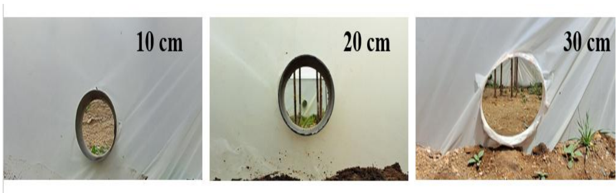
Figure III. 11: Inlet size configurations used in the experimental setup.
