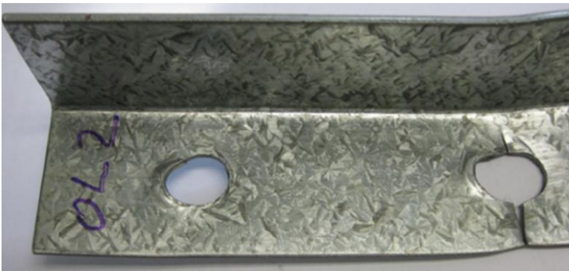
Figure 2-11. Net section tension failure [154]
