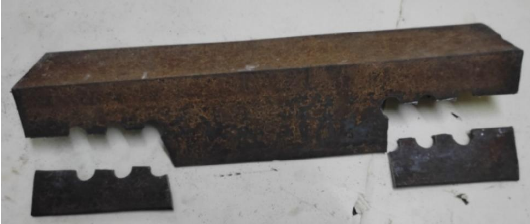
Figure 2-10. Block shear failure in angle connection [153]
