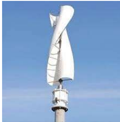
Figure I.20. Helical Darrieus Turbine Design for Enhanced Efficiency and Vibration Reduction
