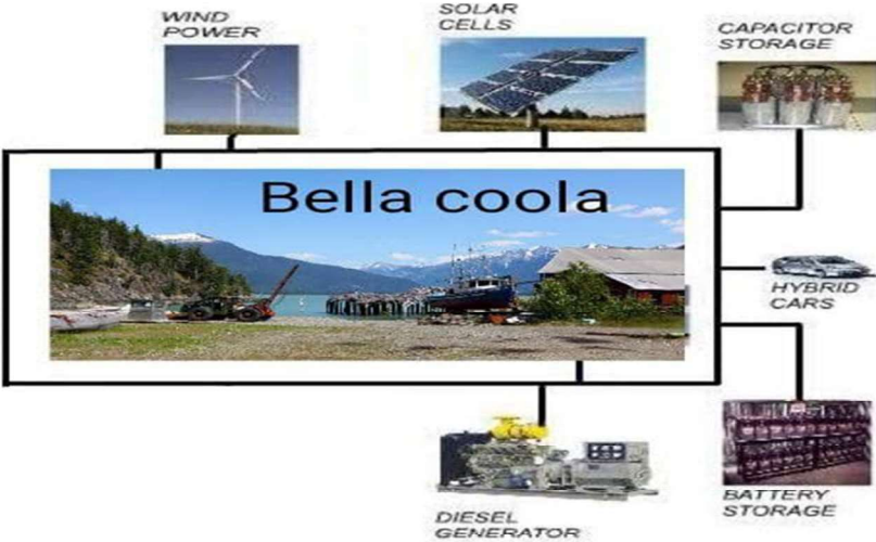
Figure I.13: Composition and structure of bella coola microgrid.
