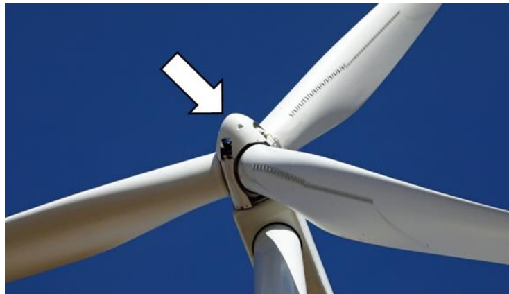
Fig. (1.10): The rotor of a wind turbine.
