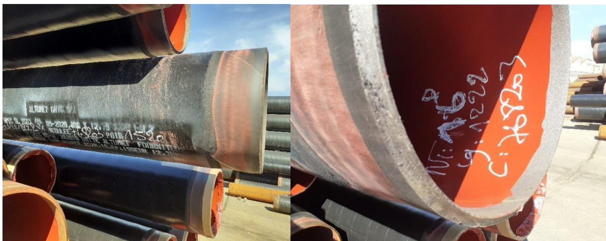
Fig.1.9 Marking of pipes a) exterior and b) interior.
