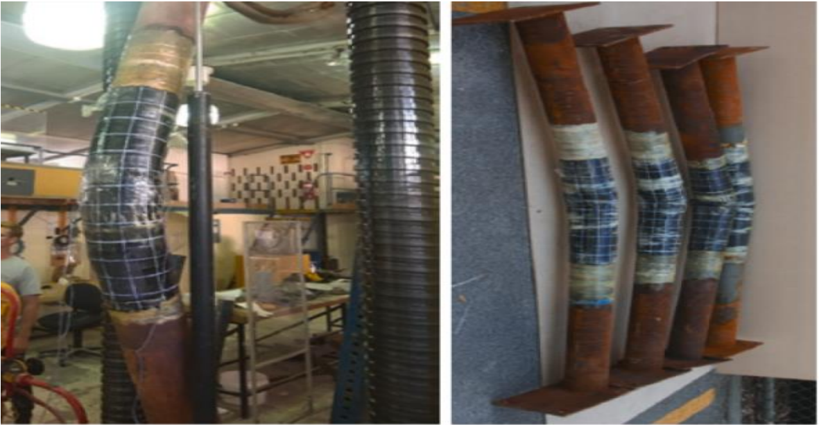
Fig.2.18 Testeafter combined axial compression [175].
