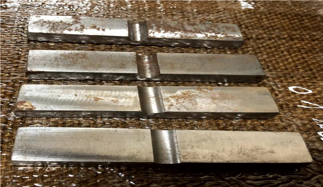
Fig.4.10 Geometry standard of semi-elliptical defects top view.
