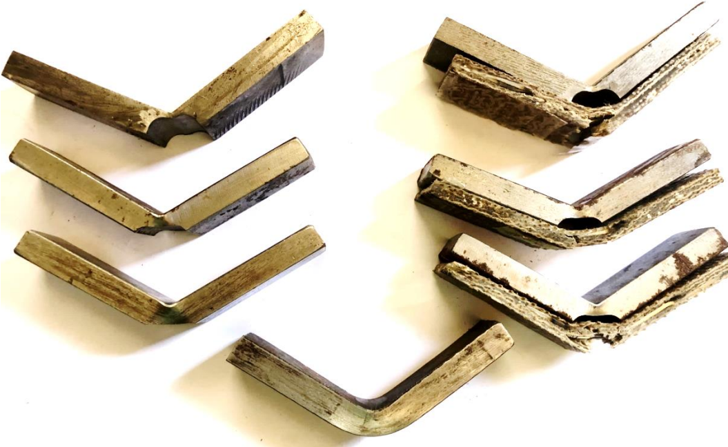
Fig.4.22 Specimen API X 52 pipeline steel test with and without repaired using the patch composite natural.
