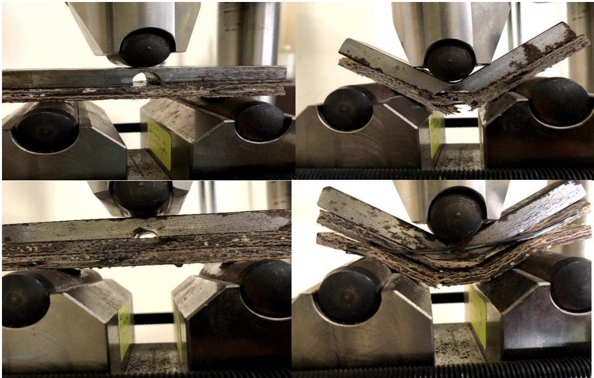
Fig.4.12 Equipment of flexural Testing and defect specimen with patch.
