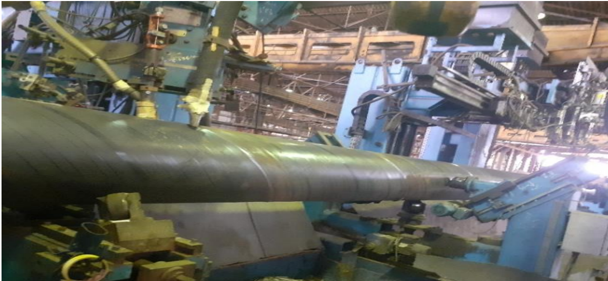
Fig.1.6 Manufacturing pipe machine in content (forming and welding).
