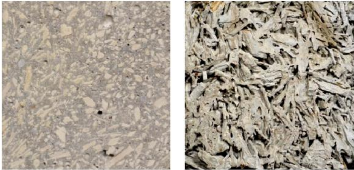
(a) Dense lightweight woodchip concrete (b) Porous lightweight woodchip concrete
