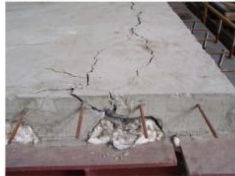
(b) Debonding at the upper flange for S2
