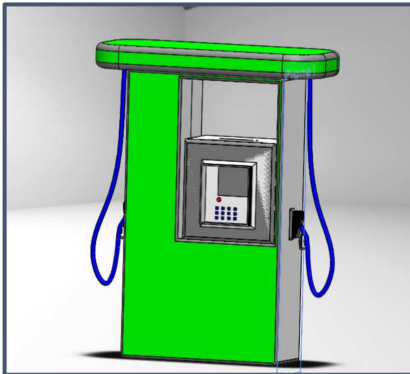
Figure (IV-10): Design of the Gilbarco Veeder Root hydrogen dispenser
