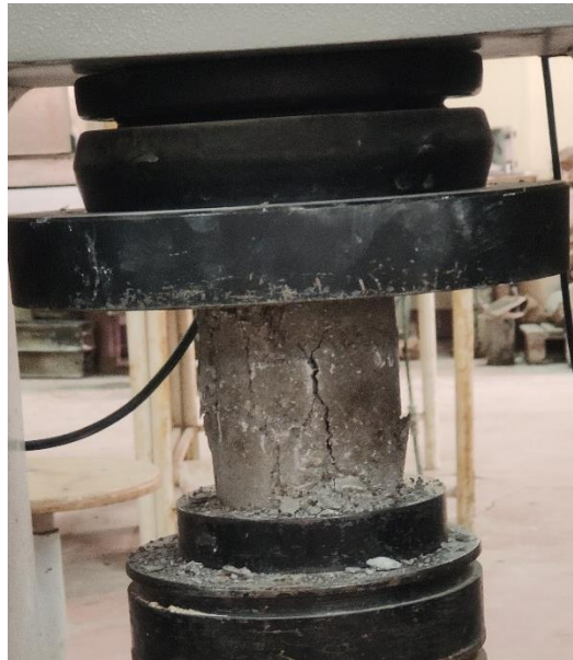
Figure 2. 25. Essai de compression simple.
