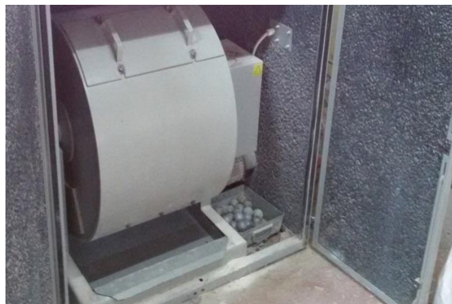
Figure 2. 10: Essai de Los Angeles .
