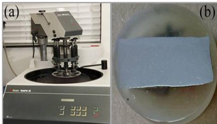
Figure II.14. Metallographic preparation of the specimens; (a) STRUERES ROTOPOL-35 polisher, (b) specimen after polishing.
