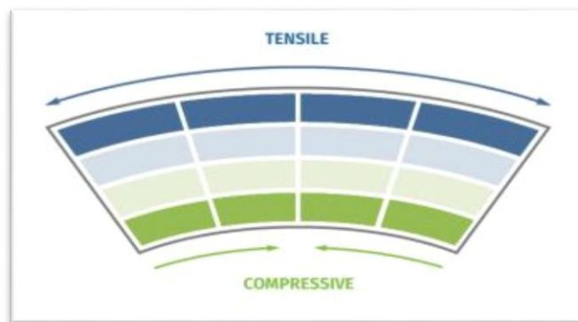
Figure I.6. Formation of tensile and compressive stresses on a bent sample
