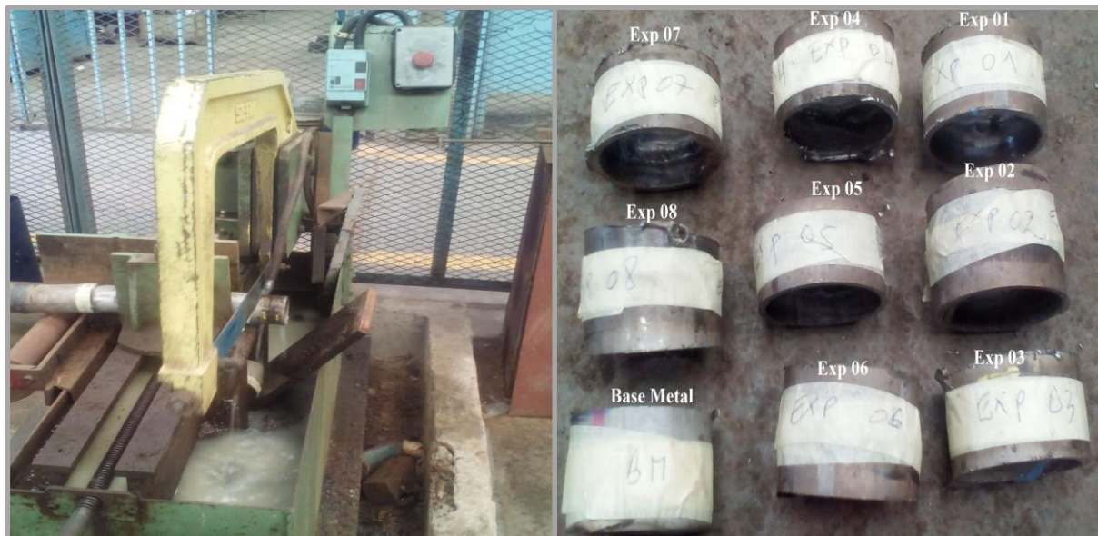
Figure II.2. Cold cutting of samples by an automatic saw
