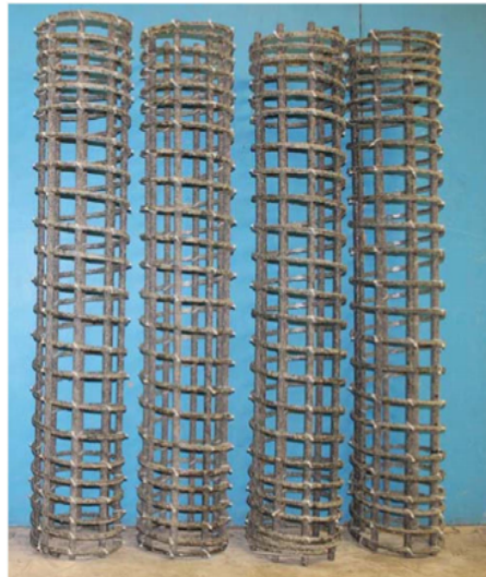
Figure I.25: CFRP cage assembly (Mohamed and Benmokrane 2014).
