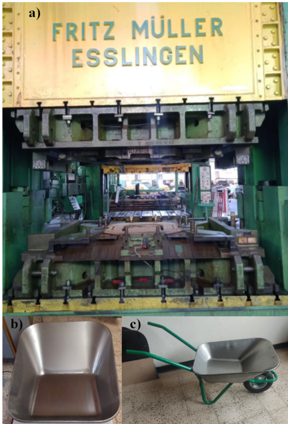
Figure 3-3 : a) BZE1600-32 Press b) Semi finished wheelbarrow tray product, c) Final product [28].
