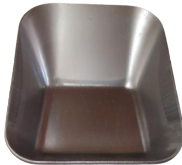
Figure 3-7: Trimming and bending operation for the wheelbarrow tray.
