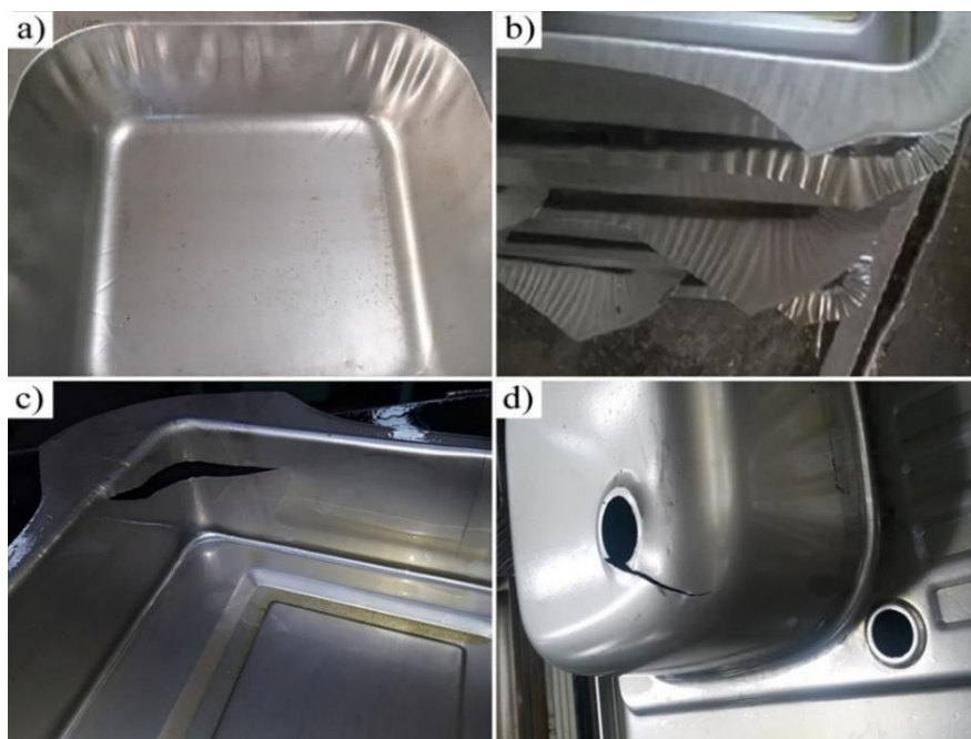
Figure 1-6 : Deep drawing defects: Wrinkling (a,b), Rupture (c,d).
