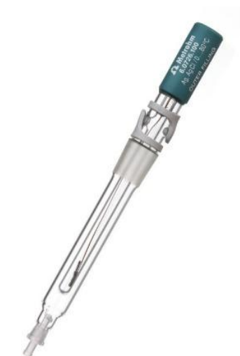
Figure 3.2 Ag/AgCl/3.0 M KCl (Mettrom electrode: 6.0726.100)
