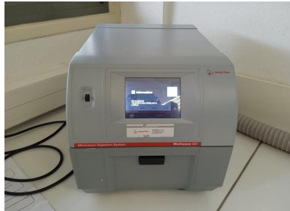
Figure II.8: Microondes Multiwave GO (Anton Paar).
