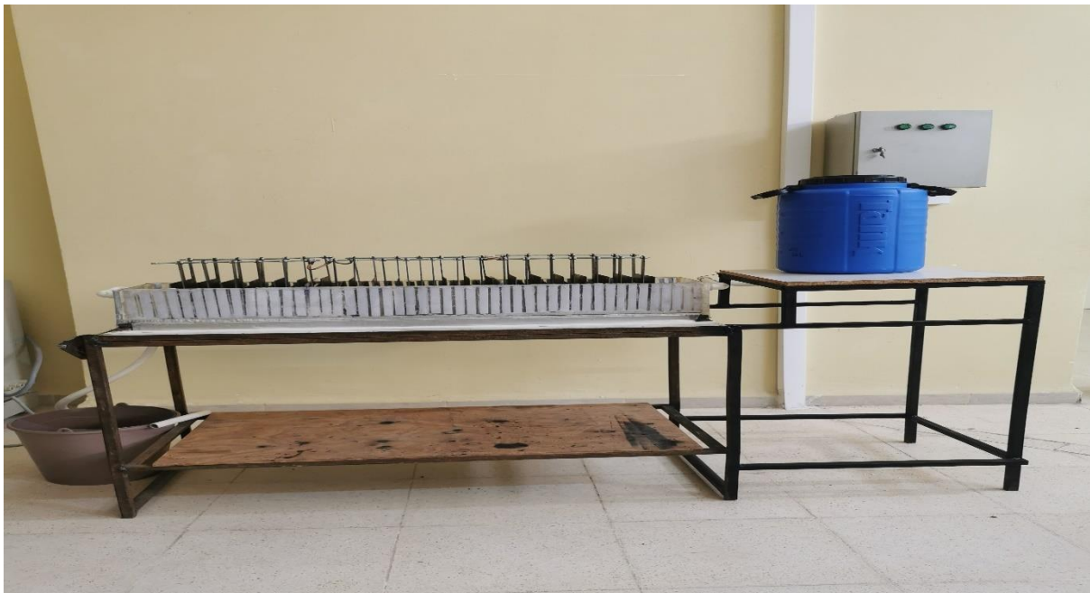
Figure (III.2) : System de l'électrocoagulation.
