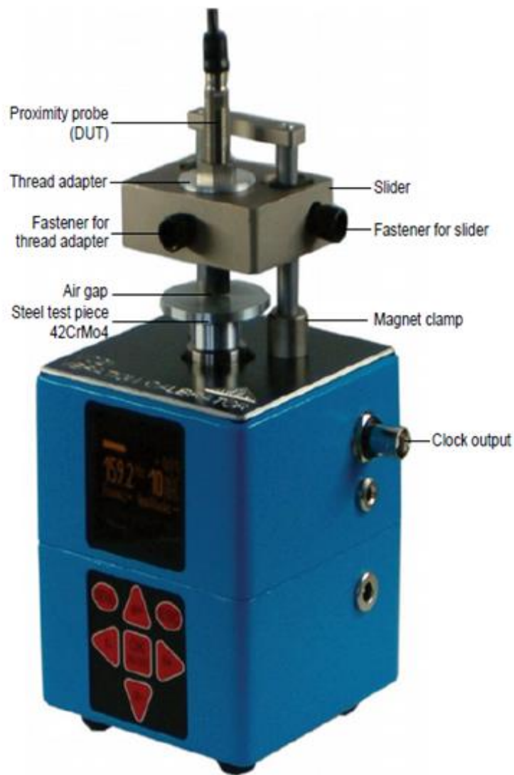
Figure 21: Vibration Calibrator VC 21D with clamping devices.
