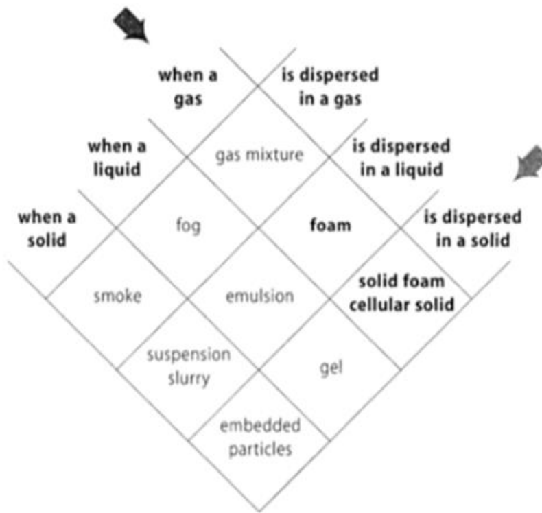
Figure 14: Dispersions of one phase into a second one. Each phase can be in one of the three states of matter [65]
