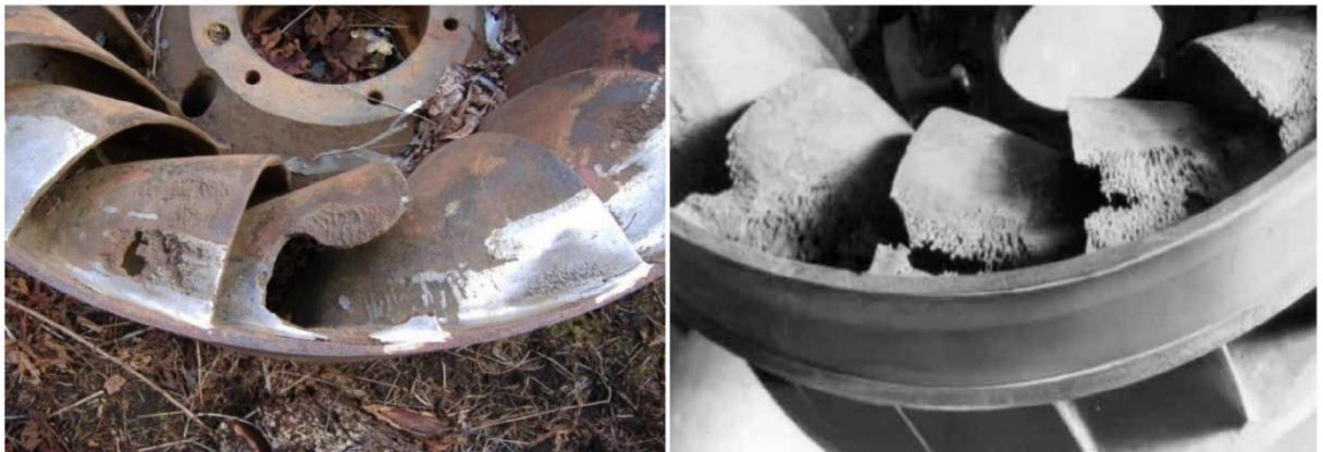
Figure 2: Francis Turbine Cavitation Damage (A) [6] and (B) [5].
