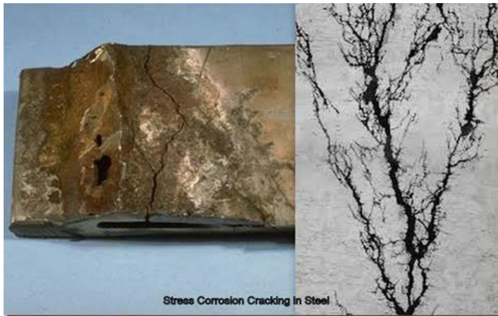
Figure II. 11: stress corrosion cracking [72]
