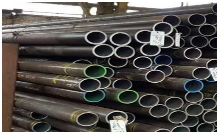
Figure I. 13:X80 Carbon Steel Pipeline [30]
