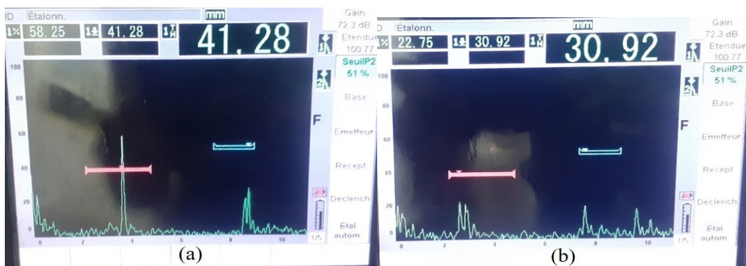
Figure III.9. Condition(2), (a)avec bourrelet et(b) sans bourrelet
