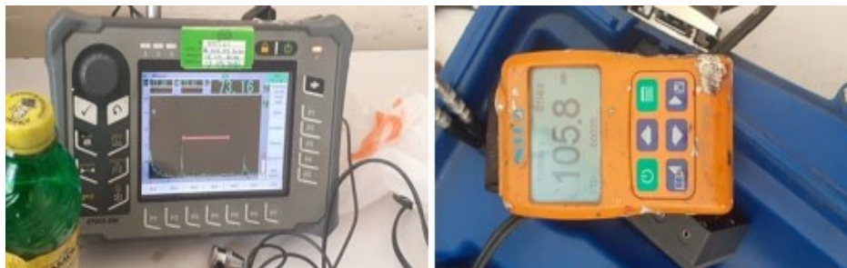
Figure II.11. Poste ultrasons type impulsion
