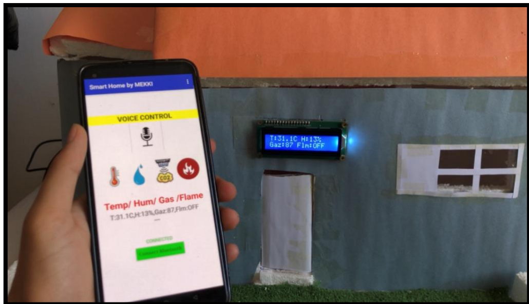
Figure (IV.22): Implemented tasks of a Mobile Application for Real-Time Control and Monitoring of Smart Home Systems.
