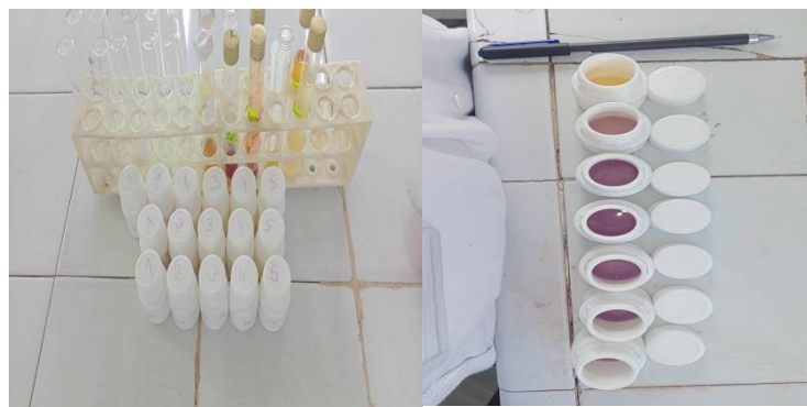
Figure 83: DPPH incubation of sage, fenugreek and date seeds extracts at different concentrations.
