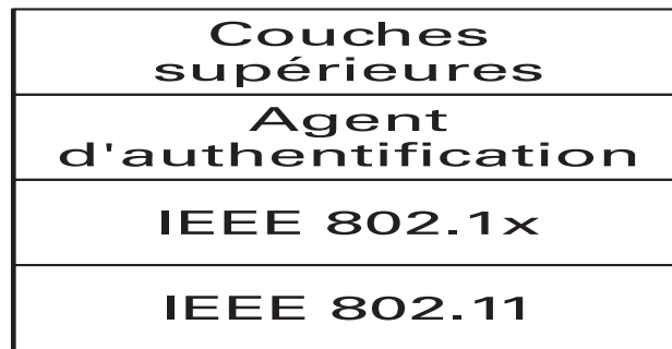
FIGURE VI.8 – Architecture IEEE 802.11 incorporant IEEE 802.1x.
