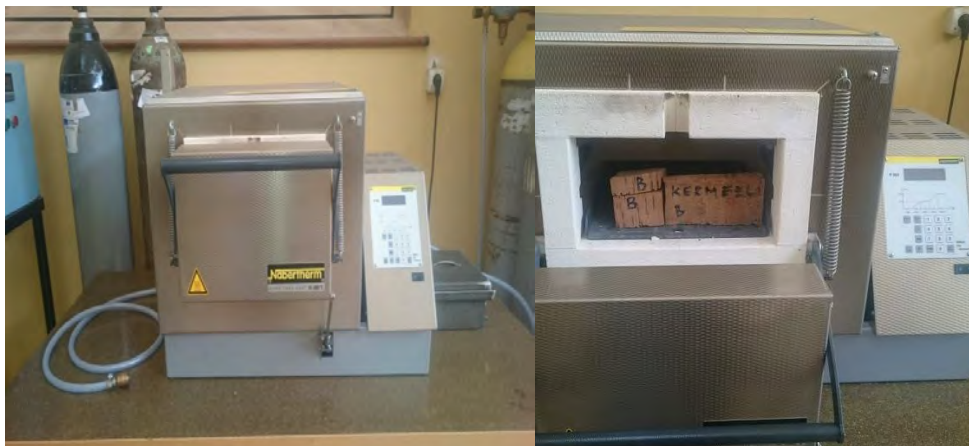
Figure II.5 : Four de THT 'L.M. Ecole Militaire Polytechnique'
