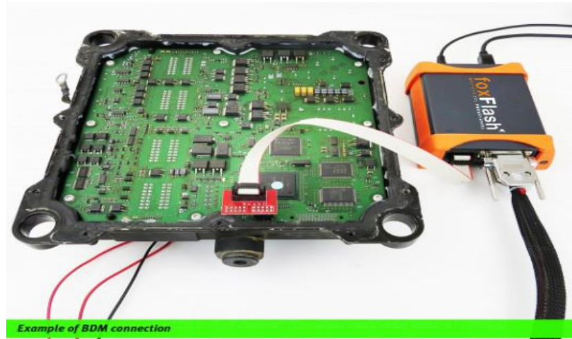
Figure 4.4: Mode BDM (Background Debug Mode) [6]
