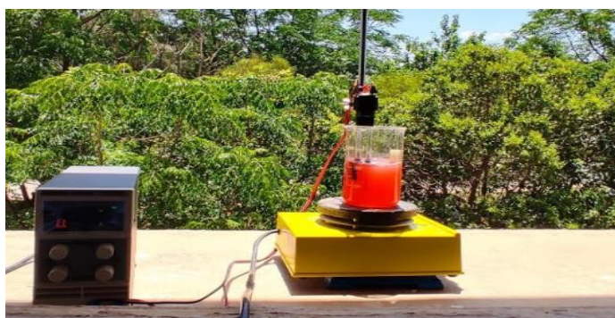
Figure III-E-3. experimental set-up for electrophotocatalysis of methyl orange under solar irradiation
